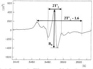
Fig. 1. Representative EPR spectrum of 5-nitroxyl stearate (5-NS). T-tensor measurements from which the order parameter is calculated and the signal amplitude of the central resonance line  $(B_0)$  are indicated. The concentration of the spin probe is 1.6  $\mu$ M in the mitochondrial plus synaptosomal suspended in calcium-free Krebs buffer.
